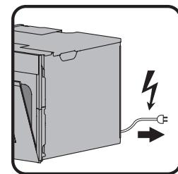
Connect cable to connecting terminals in accordance with connection plate
